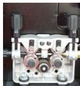
(10) Install a U groove drive roller of the size for the diameter wire being used.
