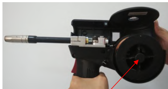
(10) Place a spool of wire onto the Spool holder.
