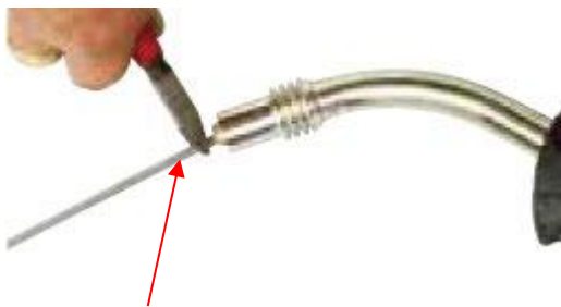
(7) Snip the liner off 3mm past the end of the torch neck.
