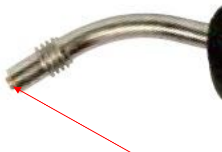
(1) Remove mig torch front end parts.
