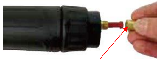
(2) Remove the liner retaining nut.
