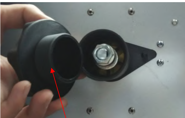
(1) Remove the spool retaining nut.
