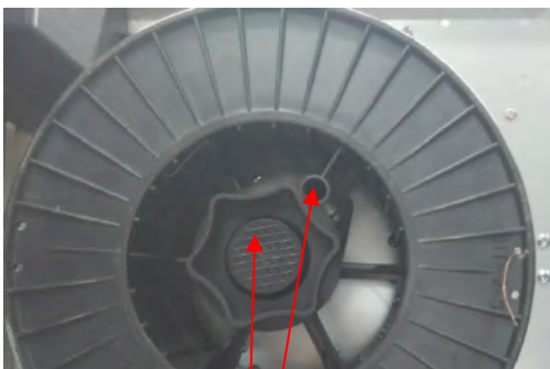
(1) Remove the spool retaining nut.
