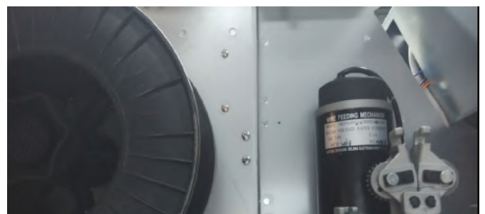
(2) Note the tension spring adjuster and spool locating pin.
