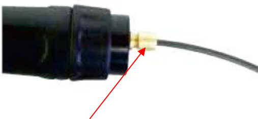
(6) Push the liner firmly into the torch lead and tighten the liner retaining nut.
