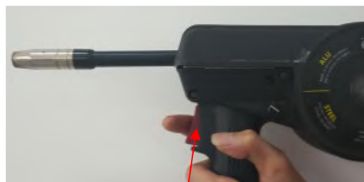
(12) Pull the trigger to drive the wire through the neck until it exits the contact tip holder.
