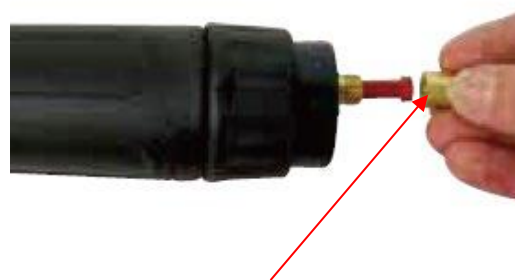
(2) Remove the liner retaining nut.
